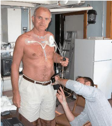
Fig. 2. Example of noninvasive physiological sensors (Nexan Ltd.), which can transmit data wirelessly via an attached PDA. Measures 2-lead electrocardiogram, pulse oximetry, heart rate, respiration rate and temperature.
