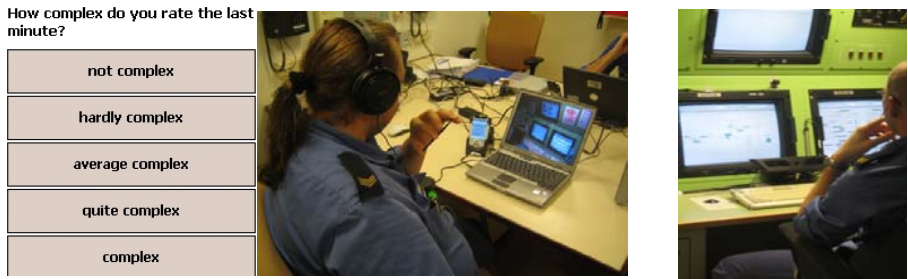
Fig. 3. Operator scoring complexity and effort during video replay of the just performed scenario (left and middle). Measuring pupil dilation (right).
