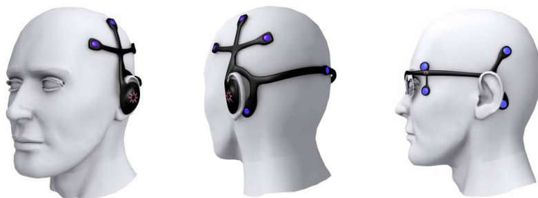
Fig. 6. Two concepts for a sensor harness suitable for operation in a C2 environment
